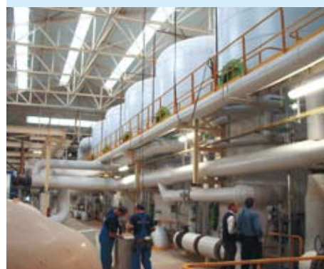
Sugar Factory in Belgium Evaporation station with 8 effects
