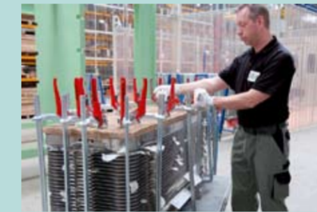
9. Tensioning the plate pack with subsequent accelerated setting of the adhesive in a furnace
