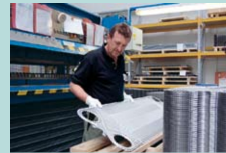
7. Alignment and any necessary repair of the gasket groove
